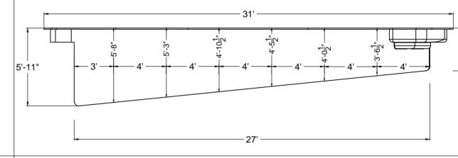
The bottom configuration shown conforms with current ISPSC & ANSI / APSP / ICC suggested minimum standards for pools <u>NOT</u> approved for diving.
