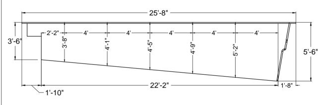
The bottom configuration shown conforms with current ISPSC & ANSI / APSP / ICC suggested minimum standards for pools NOT approved for diving.
