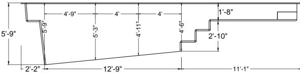
The bottom configuration shown conforms with current ISPSC & ANSI / APSP / ICC suggested minimum standards for pools <u>NOT</u> approved for diving.
