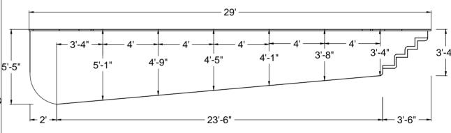
The bottom configuration shown conforms with current ISPSC & ANSI / APSP / ICC suggested minimum standards for pools NOT approved for diving.
