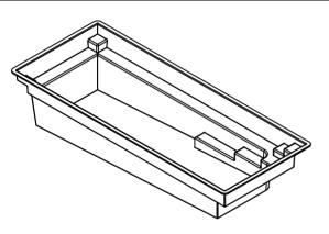
The bottom configuration shown conforms with current ISPSC & ANSI / APSP / ICC suggested minimum standards for pools NOT approved for diving.
