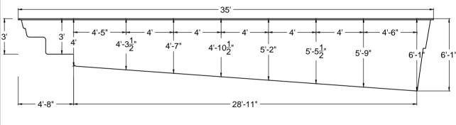
The bottom configuration shown conforms with current ISPSC & ANSI / APSP / ICC suggested minimum standards for pools <u>NOT</u> approved for diving.
