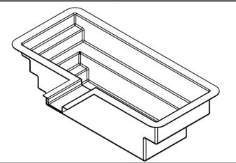
The bottom configuration shown conforms with current ISPSC & ANSI / APSP / ICC suggested minimum standards for pools <u>NOT</u> approved for diving.
