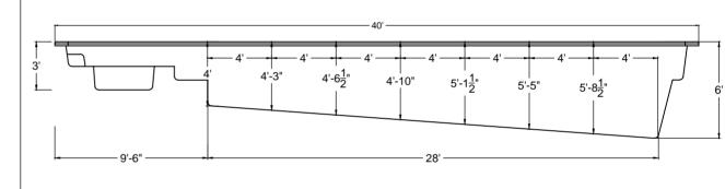
The bottom configuration shown conforms with current ISPSC & ANSI / APSP / ICC suggested minimum standards for pools NOT approved for diving.
