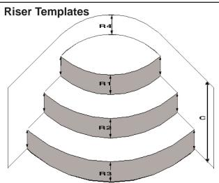
With these wall foam templates, please measure the riser heights. If the heights are not uniform, include the different measurements (right, left and center). Riser heights MUST equal the C dimension (bead to floor).
