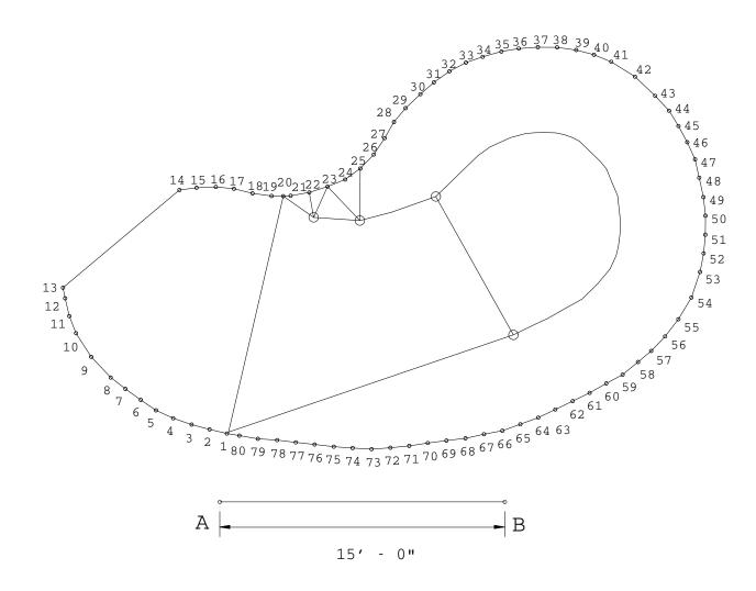
It is important to recognize at this stage the difference between the COPING perimeter and the BOTTOM OF THE WALL perimeter. In some instances you will find that the walls are not vertical. This can be determined in two ways:
