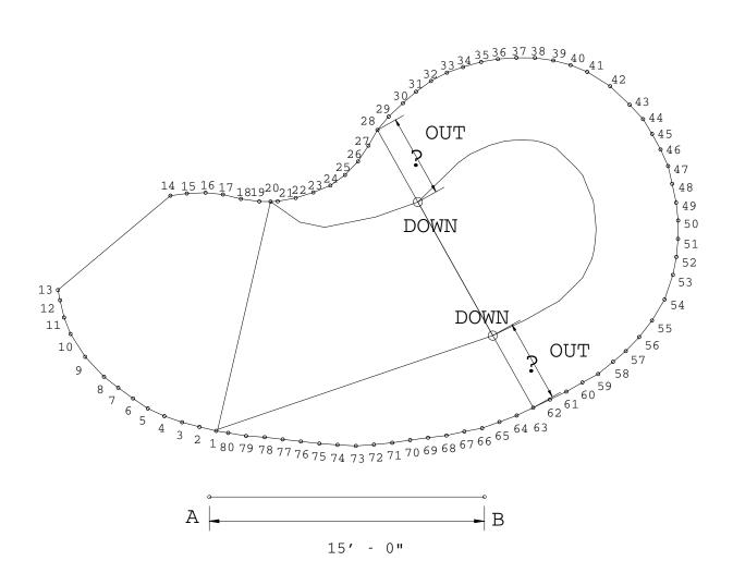
Now the rest of the pad must be located using two points on the perimeter for every internal point. In this example, we will be finding internal points U, V, W, X, Y, and Z. Here's how...
