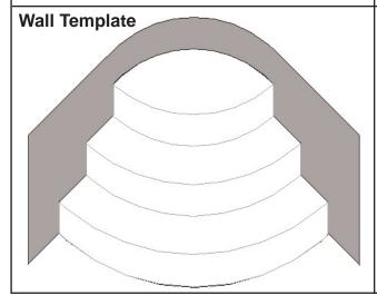
This wall foam template is not always necessary, but in some cases we may require it for the manufacturing of the staircase.
