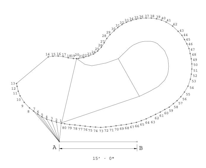
With the 100' cloth tape, move to stake "B" and measure from B to #1; record this measurement on the "CUSTOM LINER & SAFETY COVER ORDER FORM." Now measure B to #2, B to #3 and so on, until the last number is reached. (#80 in this example.) Check your numbered progress often, to make sure you do not skip any.
