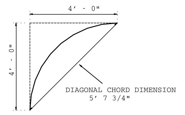
NOTE: The size of the radius is not the perimeter value or the diagonal chord dimension.
