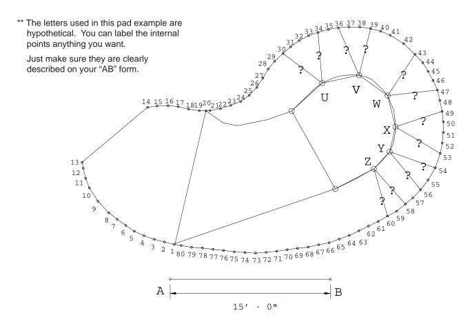
If your pool has a long slope that does not go from the shallow break STRAIGHT to the pad corner, interior dimensions will be necessary. In this example, if you are looking from shallow end to the deep end, the left side of the long slope is curved and the right side is straight. For this, the left side needs to be measured and the right side does not. The left side needs to be measured in the same way you measured the points around the deep end pad.
