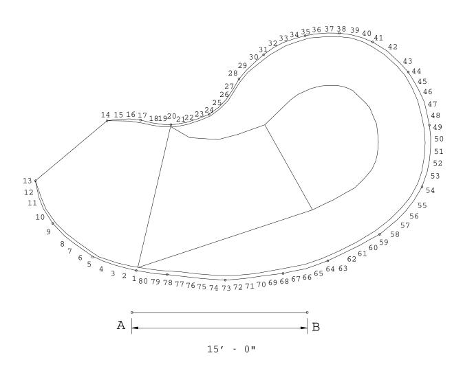
Use a plumb bob to hold over the bottom of the wall. Align the plumb bob straight out from a perimeter point. Now measure from your perimeter point out to the plumb bob line. Do this about every 3 to 4 points, depending on how close together they are. Remember to keep track of the perimeter numbers you are using and the out distances.
