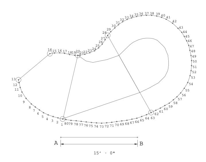
With the 100' cloth tape, start with stake "A" and measure from A to #1; record this measurement on the "CUSTOM LINER & SAFETY COVER ORDER FORM." Now measure A to #2, A to #3 and so on, until the last number is reached. (#80 in this example.) Check your numbered progress often, to make sure you do not skip any.
